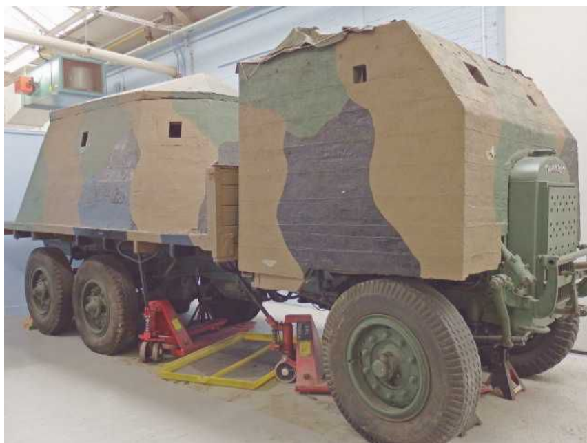
BELOW: Thornycroft Bison. A concrete pillbox on the back of a lorry with concrete cab, and a good example of the many local make-shift British vehicles constructed to compensate for the loss of BEF equipment at Dunkirk.
