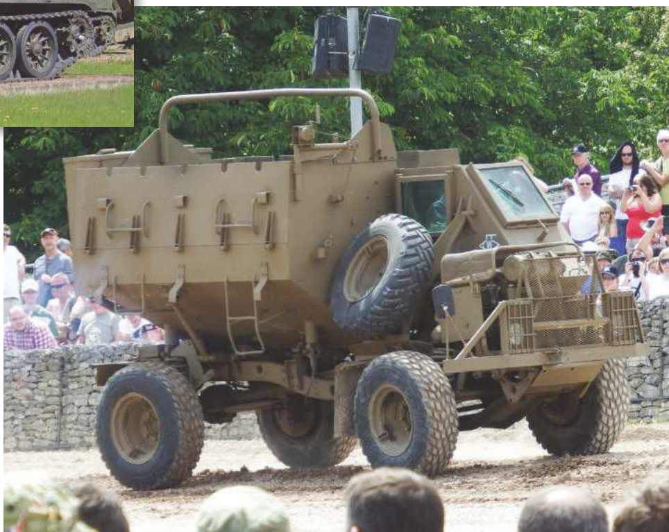
BELOW: The awkward-looking Buffel, at Tankfest is not a beauty. Entering service with South Africa in 1978 in its Bush Wars, it was the first mine protected vehicle with a raised crew compartment shaped to deflect mine blasts.
