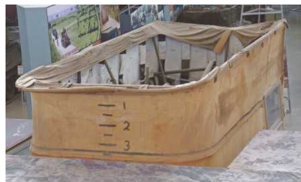
BELOW: Sherman DD, now well known as one of the 79th Armoured Division Funnies but may not have been so amusing to a beach defender seeing these emerge from the sea as in this overhead view at Bovington. One of several amphibious tanks designed by innovative Hungarian engineer Nicholas Straussler, many of his military vehicles and equipment inventions were of quirky appearance.
