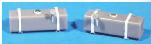
ABOVE: Fuel tanks showing correct length of filler pipe, support fillets, correct location of supports, new straps and beefed up fuel line fitting.
